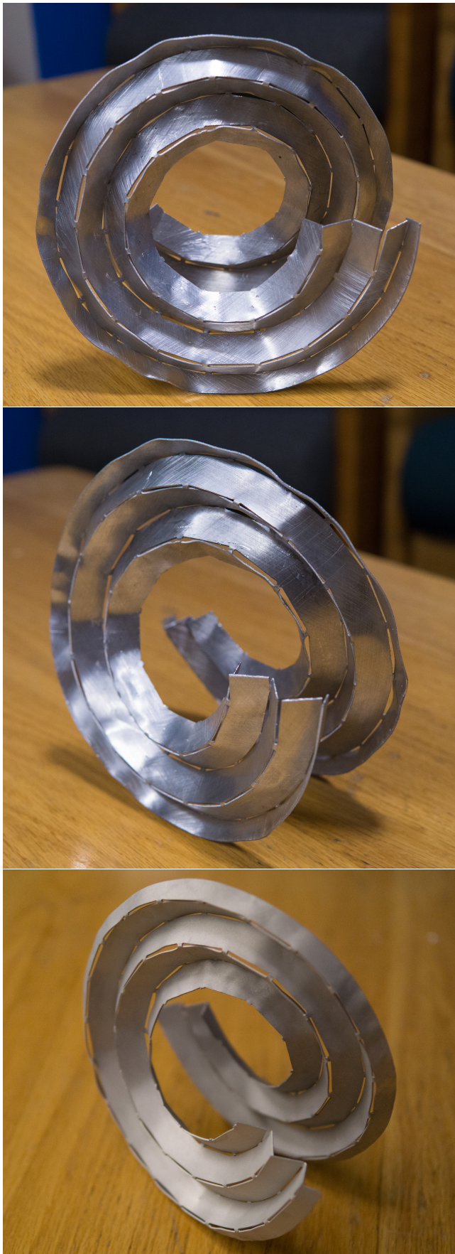
(a) The aesthetics were significantly improved with a bit of extra care bending back wrinkled sections and sandblasting the piece.
