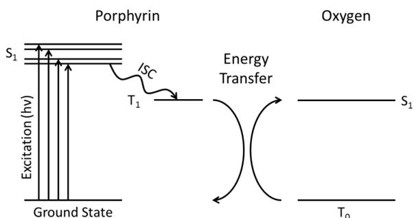
Figure 2: Graphical depiction of the photophysical mechanism behind singlet oxygen production in PDT.
