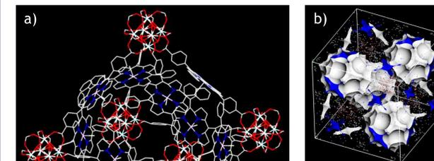
Figure 5: Results of structure determination studies on MOFs. In (a), from single-crystal X-ray diffraction patterns, we see that the MOF takes on an octahedral repeat unit, and based on PLATON calculations (b), we have calculated 70% pore-accessible volume. In (c), PXRD patterns for MOFs, show that Mn MOF has at least two phases, and Zn MOF is isostructural to one of the phases of the Mn MOF. Moreover, the non-metallated MOF is not very crystalline. The common phase is shown in (a).
