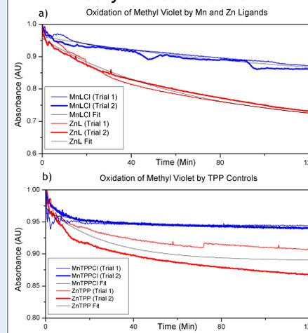
Figure 4: Results of PDT representative studies in methyl violet oxidation, showing that ZnL was most effective. This was predicted due to Zn's higher  $T_1$  state lifetime and the carboxylic acid groups of the ligand increasing quantum efficiency.
